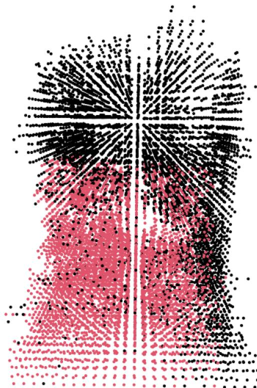
Figure 2: Resulting point cloud after a completed simulation (used parameters: *time* = 10, *range* = 2, *wind direction* = "N", *strength* = 1, *res* = 1, *prob* = 0.5, *fill threshold* = 30). Red points represent voxels which have burned, black points are unburnt voxels.
