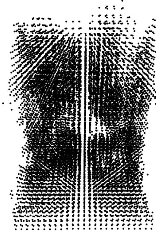
Figure 1: Example of a voxelized terrestrial laser scan with each point representing a voxel which exceeds a fill threshold
